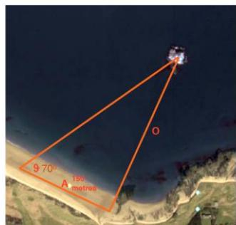
The basic method has been used in mapping for centuries. Suppose we have a remote island some distance off shore.
